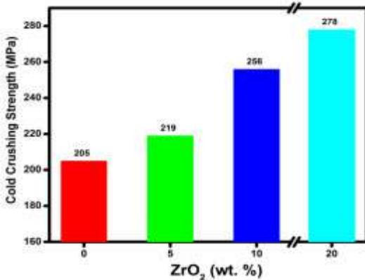
**Figure 2.** Cold Crushing Strength vs. ZrO<sub>2</sub> (wt. %)
