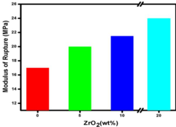
**Figure 4.** Modulus of Rupture vs. ZrO<sub>2</sub> (wt. %)
