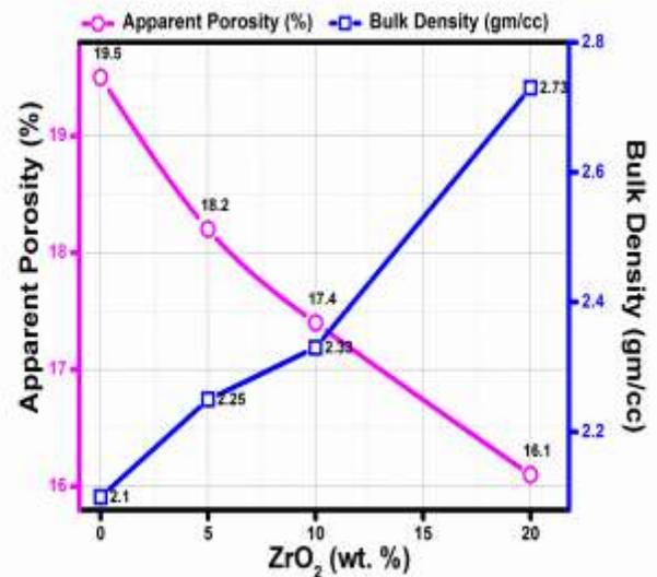
**Figure 1.** Bulk density (BD) and apparent porosity (AP) measurement
