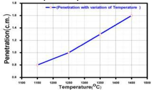
Figure 10. Penetration vs. Temperature
