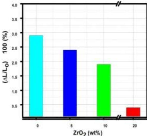
**Figure 5.** Permanent Linear Change vs. ZrO<sub>2</sub> (wt. %)
