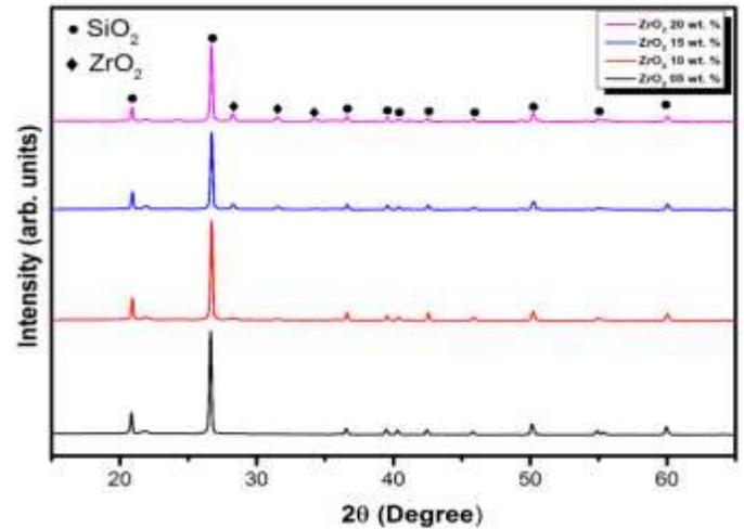
**Figure 3.** X-Ray Diffraction plot of prepared SiO<sub>2</sub>-ZrO<sub>2</sub>
