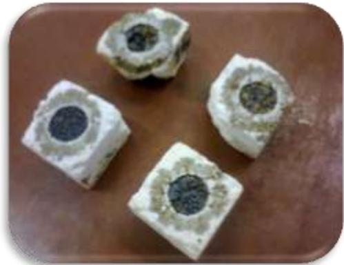
Figure 8. Sample after penetration of slag
