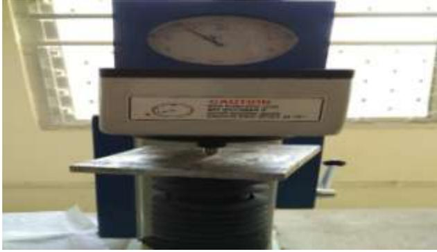
**Fig.2.3 Rockwell Hardness Testing Machine**
