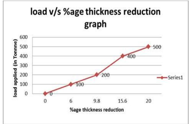
**Fig.3.1 Load V/S Percentage Reduction in Thickness**
