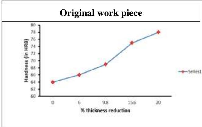
Fig. 3.2 hardness vs. percentage thickness reduction
