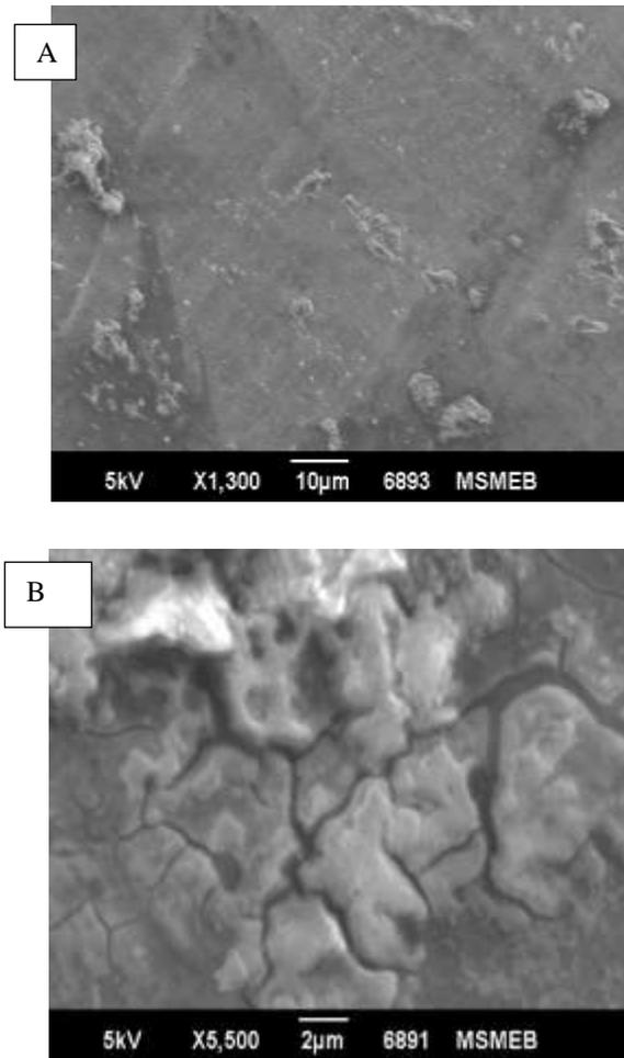
Fig 4.2 SEM images of Cu-10%Cr composite at 400X in different view angle
