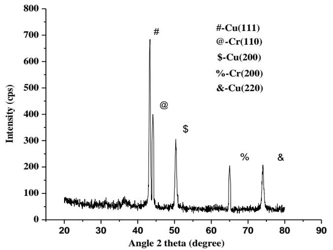
Fig 4.5 XRD pattern of Cu-3%Cr composite
