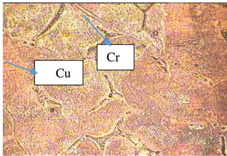
Fig 4.1 Microstructure of (a) Cu-3%Cr at 400X
