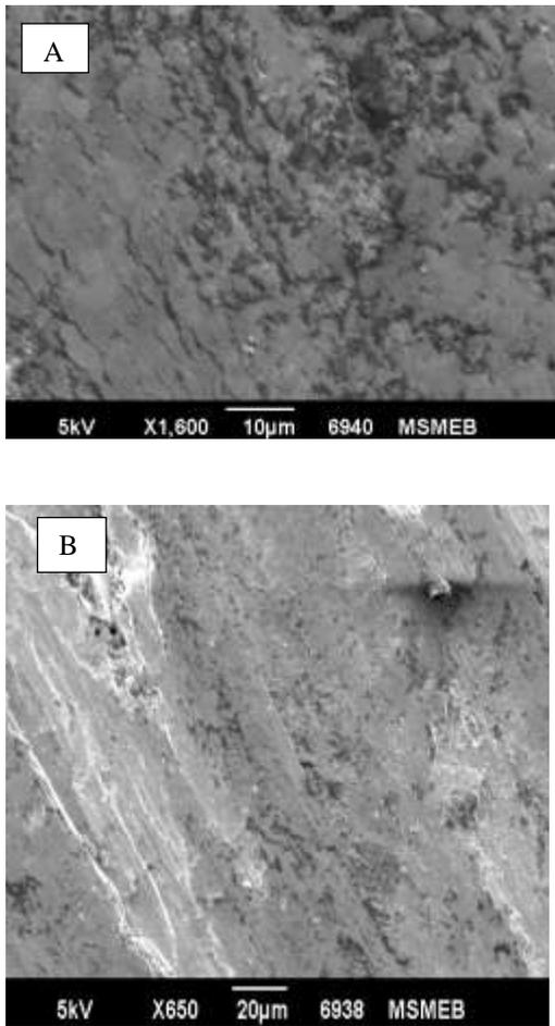
Fig. 5.3.1 SEM image of worn surfaces of Cu-10%Cr at 10N at (a) 300 rpm and (b) 400 rpm
