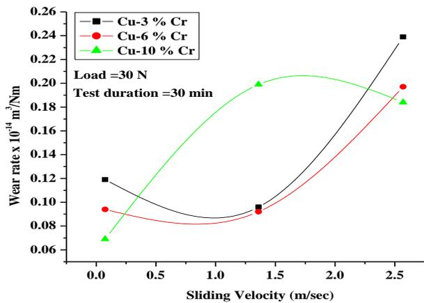
Fig.5.2.2 Variation of wear rate with sliding velocity
