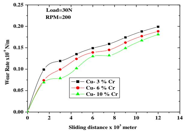
Fig. 5.1.2 Variation of wear rate with sliding distance
