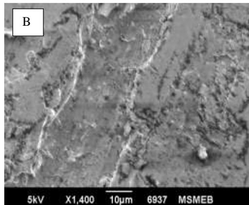
Fig.5.3.2 SEM image of worn surfaces of Cu-6%Cr at (a) 10 N and (b) 20N
