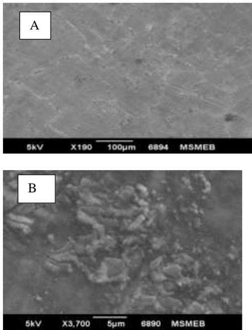
Fig 4.4 SEM images of Cu-3%Cr composite at different magnification
