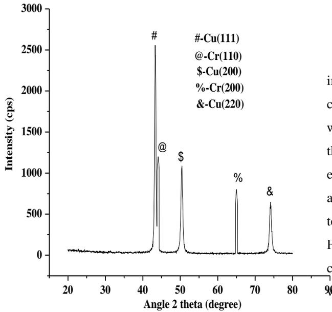
Fig 4.6 XRD pattern of Cu-6%Cr composite
