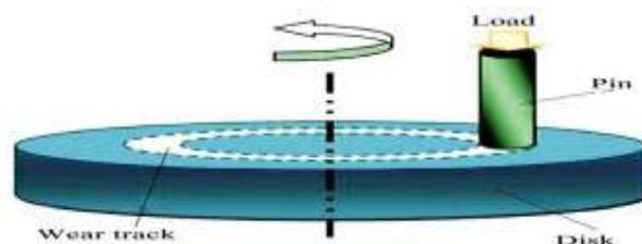
Fig. 3.5 Schematic diagram of abrasion wear test [8]
