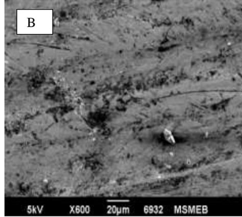
Fig. 5.3.1 SEM image of worn surfaces of Cu-3%Cr at 10N at (a) 300 rpm and (b) 400 rpm
