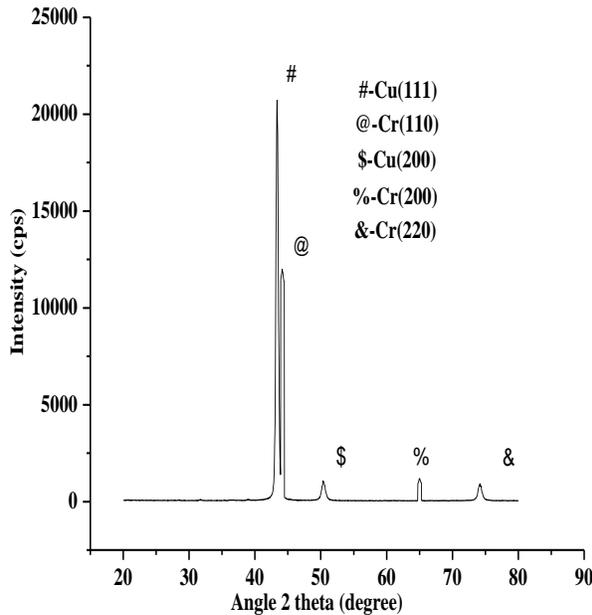
Fig 4.7 XRD pattern of Cu-10%Cr composite
