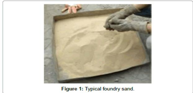
Figure 1: Typical foundry sand.
