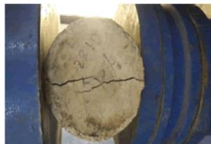
Figure 5: Failure of specimen along with wood ash.
