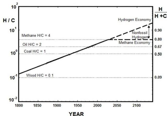
Figure 6: Decarbonization: Evolution of the Ratio of Hydrogen (H) to Carbon (C) in the World Primary Fuel Mix [24]
