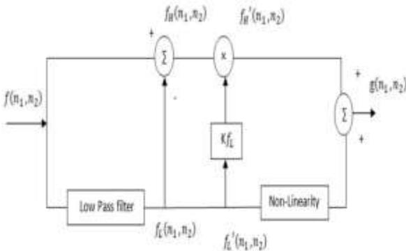
Fig. 1: Block Diagram of the Nonlinear Enhancement Method
