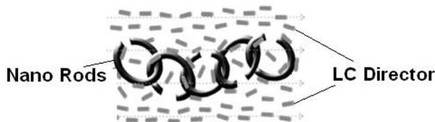
90 **Fig. 6** ZONPs (nano rods) in the nematic LC above threshold field
