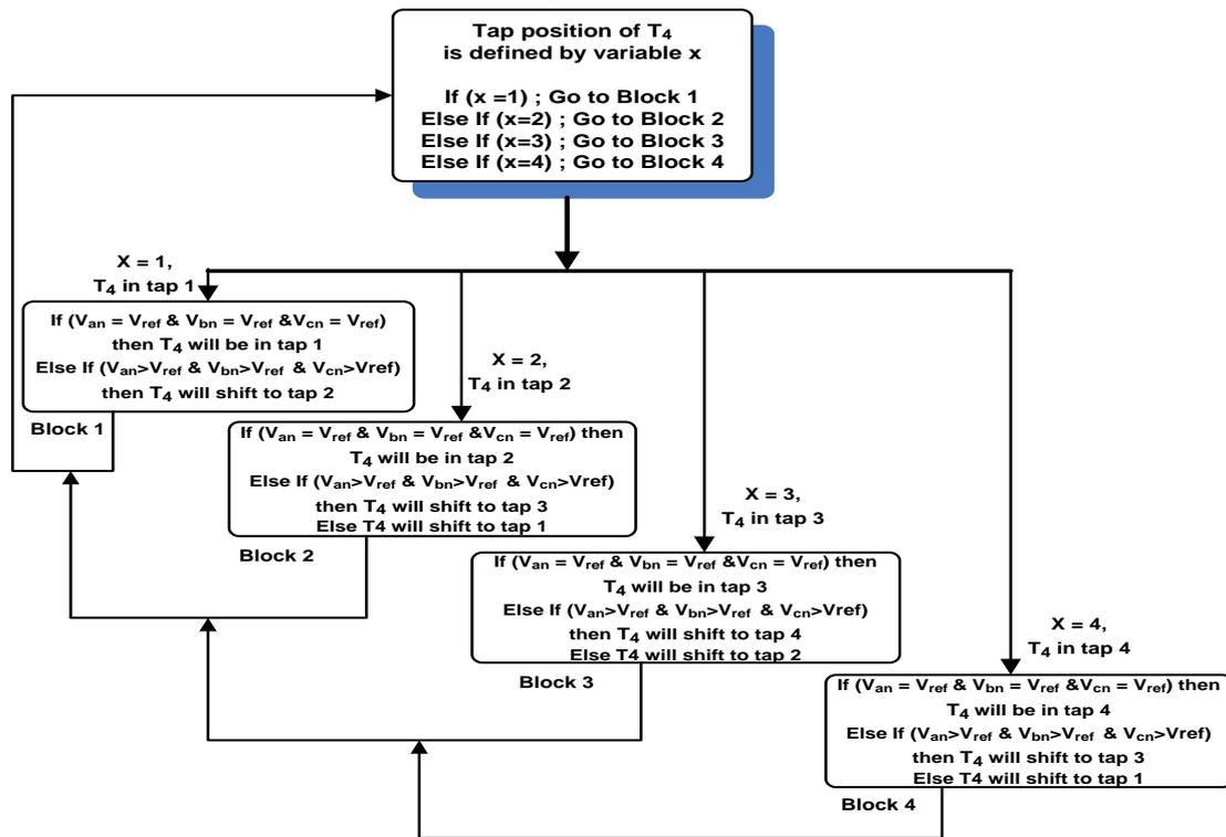
Fig. 4 Operational logical diagram of AVR
