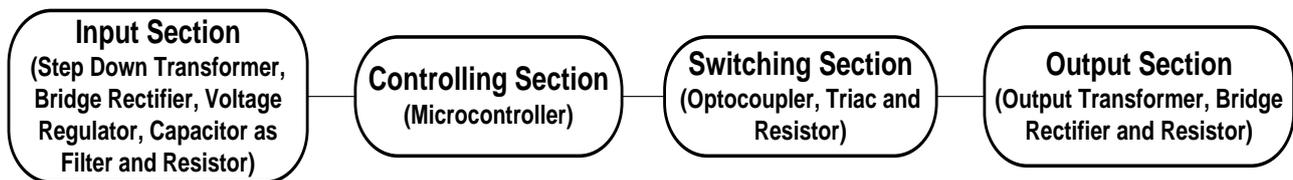
Fig. 2 Block diagram of the AVR
