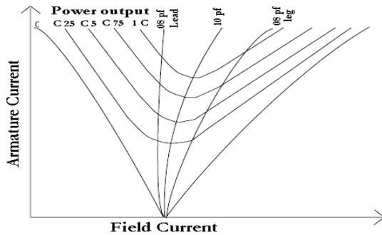
Fig. 1 V curve of alternator
