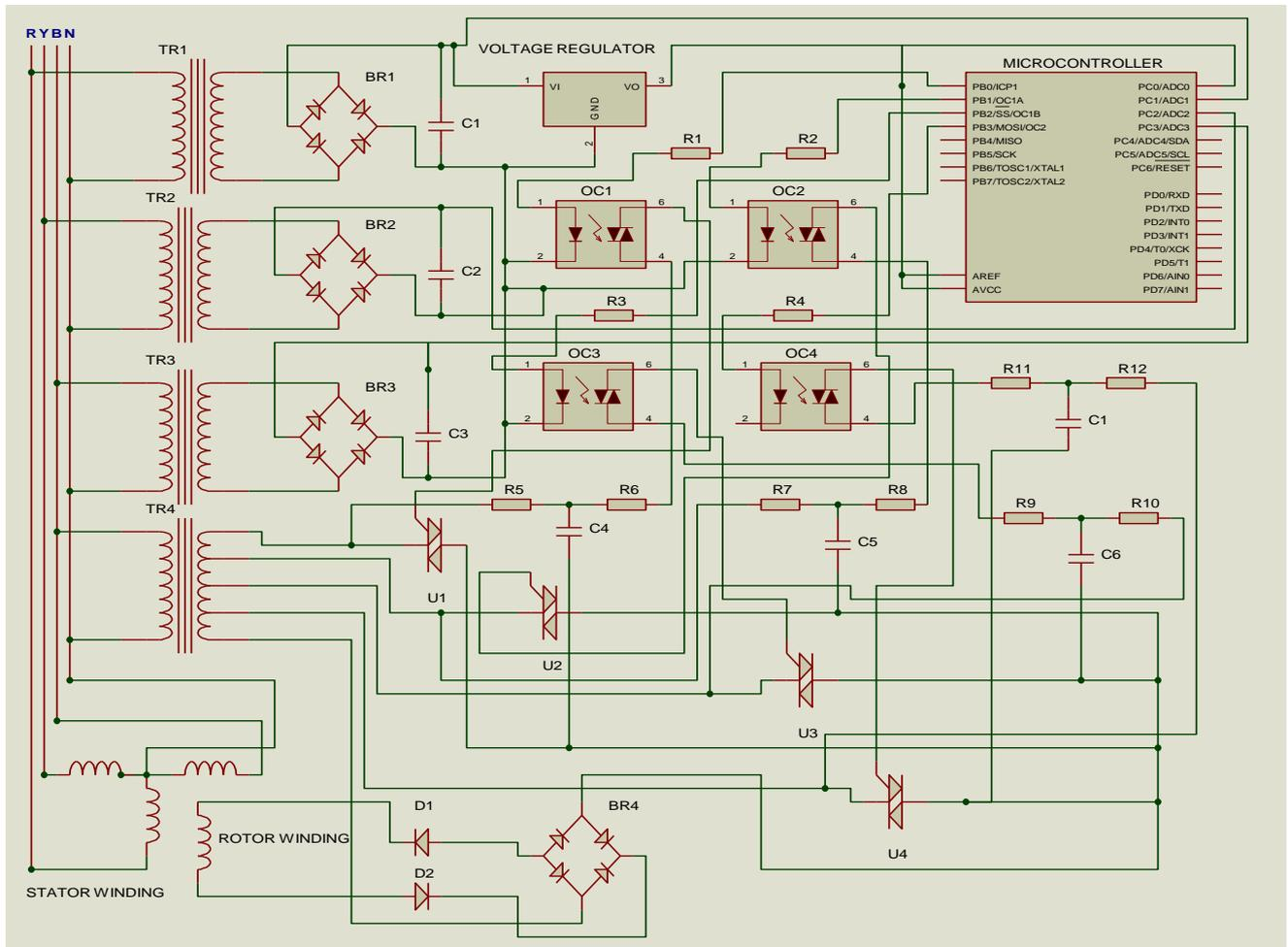
Fig. 3 Complete circuit diagram of AVR
