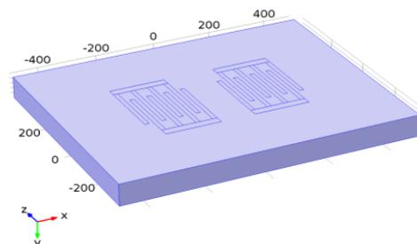
Fig. 2 Geometry of SAW delay line.
