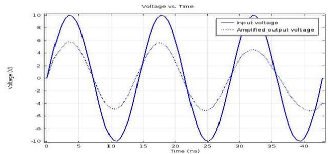
Fig. 5 Applied signal to input IDT versus recorded output potential via output IDT
