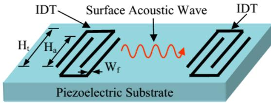
Fig.1. Basic SAW delay line [10].
